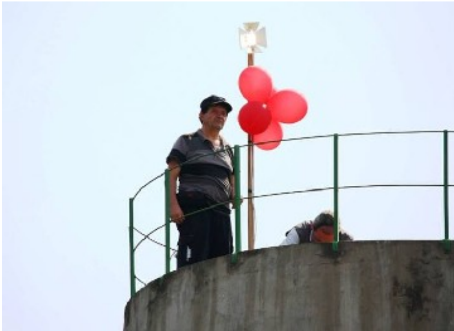
Fig. 6 – The “tools” for visual path checking (500W lamp)
